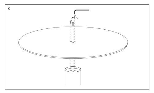
3. Mount the table base on the column with 3 (C) screws
