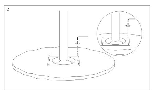
2. Lay the table top on a blanket and mount the table leg with 6 (B) screws for table top 90 cm.
