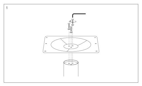
1. Mount the connection plate on the column with 3 (A) screws and 3 (A) washer
